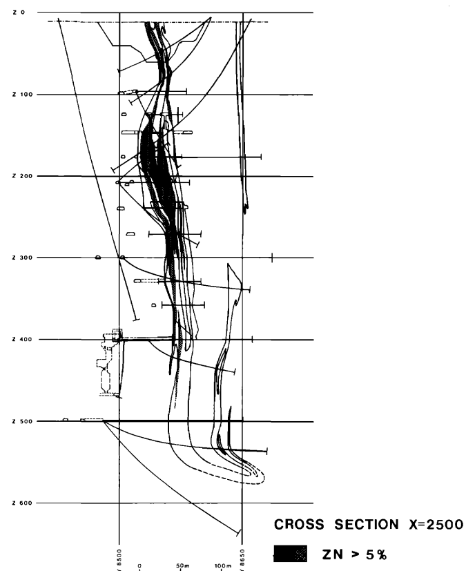
FIG. 6. Horizontal and vertical sections showing variations in the copper and zinc contents of the orebody.
